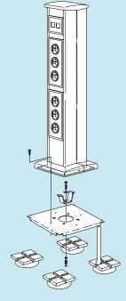
■ Mounting drawing 2 Positioning of the junction box
